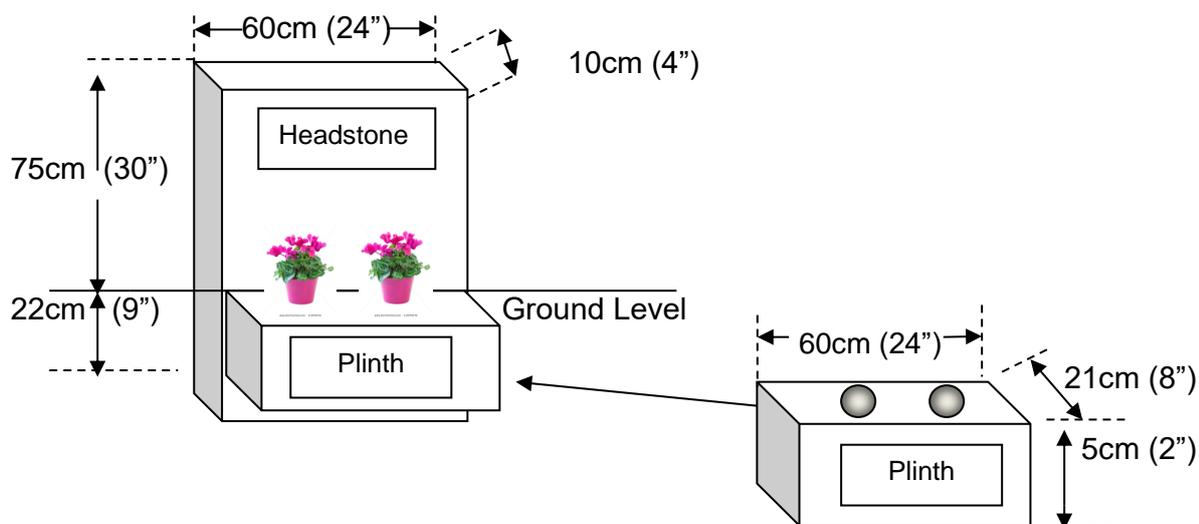
A free standing plinth, the top being level with the ground, of the same stone as the headstone may be placed in front if desired, this should be no greater than **60cm wide x 21cm deep x 5cm high (24 x 8 x 2 inches)**, and can accommodate up to two flower holders.
