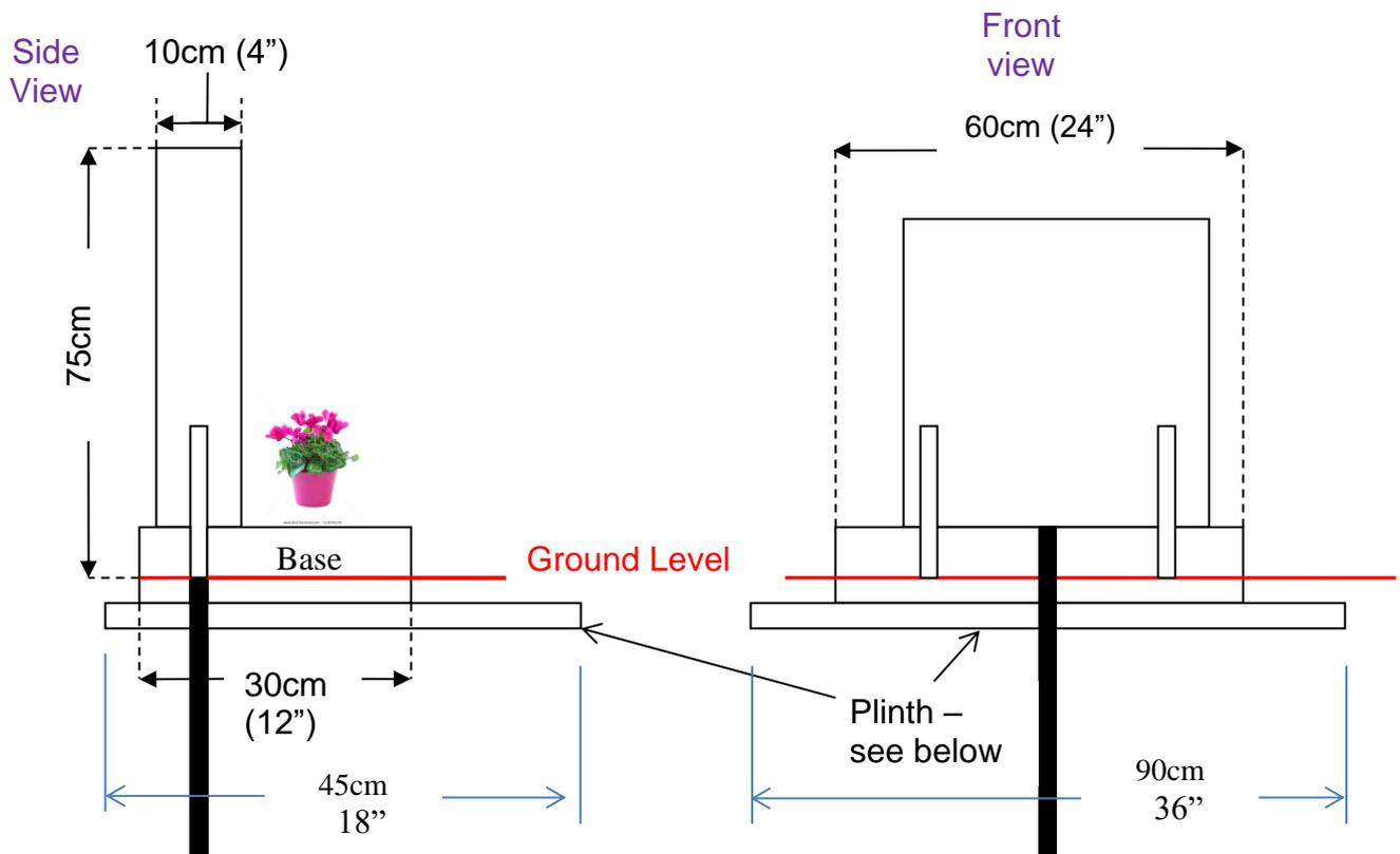
The base should be installed as per the above diagrams, and of a size no greater than **60cm wide x 30cm deep x 7.5cm high (24 x 12 x 3 inches)**. As detailed in the diagrams above, 1 inch of the base will be below ground and resting on the plinth. The base can accommodate up to two flower holders.
